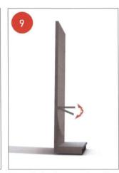
Rotate the bracket upwards until secured in a horizontal position. Brackets can also be positioned at sloping angles if desired.
