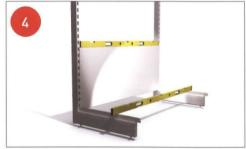
Connect both "L" shaped uprights together by fitting a back panel into the bottom "H" slots of the uprights. Now check levels are correct by adjusting the foot discs as required.
